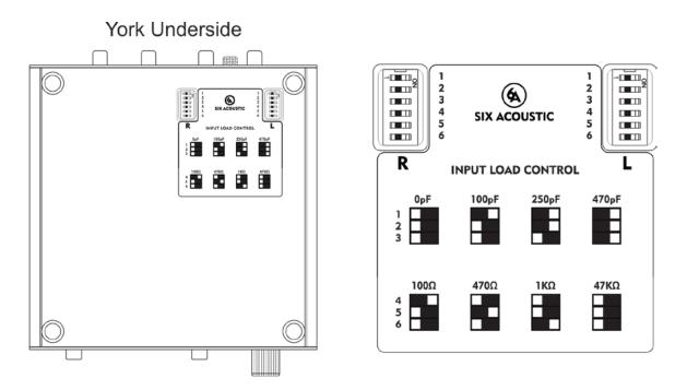
You can adjust the DIP switches on the bottom of the unit for optimal performance specific to your phono cartridge.
